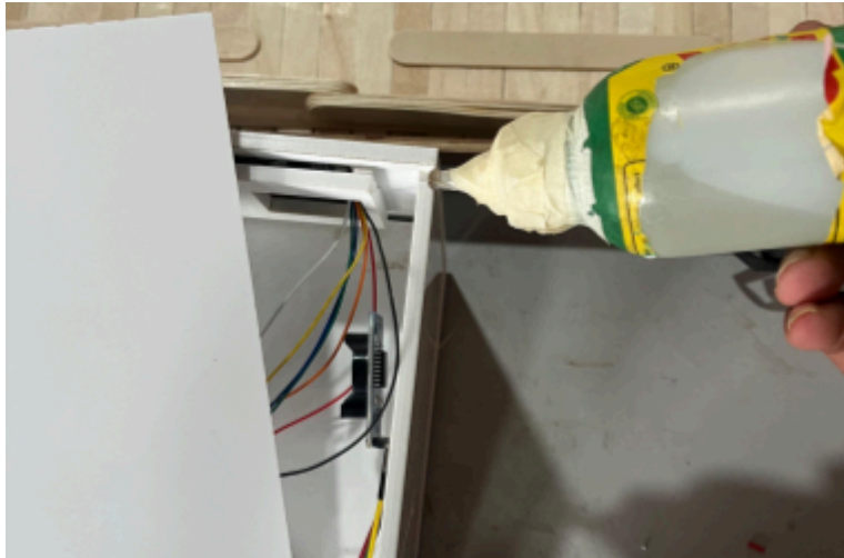
Applied glue on the top of the side panels and fixed the top panel
