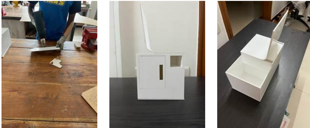
Fig. 7. Prototype fabrication and result: heat-bending the acrylic seat-and-backrest to 98° (left) and the finished 1:3 prototype from the front and above (centre, right).
